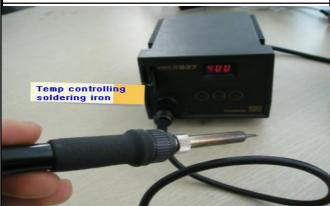
When soldering, pls set up soldering iron on  $350 \sim 400 \,^{\circ}\text{C}$ . It is best temp to solder.
