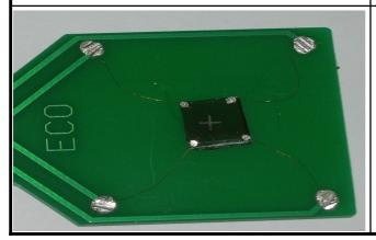
It was finished to connect wire to soldering on 4points and mounting sample on PCB board.
