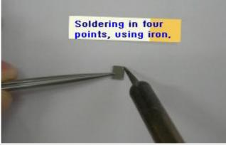
Soldering in four points using soldering iron.
