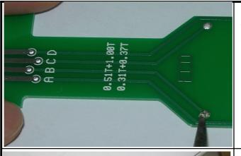
Put the soldering iron that has melted InSn compound onto four point as shown left. It 's o.k to be proceeded in the first step in advance.
